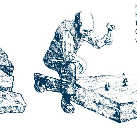
1 Using a 'jumper' (a weighted, oneperson operated drill), a line of holes was drilled approximately four inches deep and six inches apart. 2 Once the line of holes was drilled, a tapered plug called a *tare* was driven into each hole between two curved slivers of metal known as feathers. By tapping on each of the tares in turn a line of stress was formed causing the block to split along that line.
