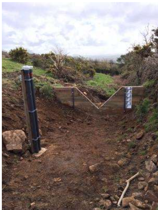
Monitoring in place- V notch weir
