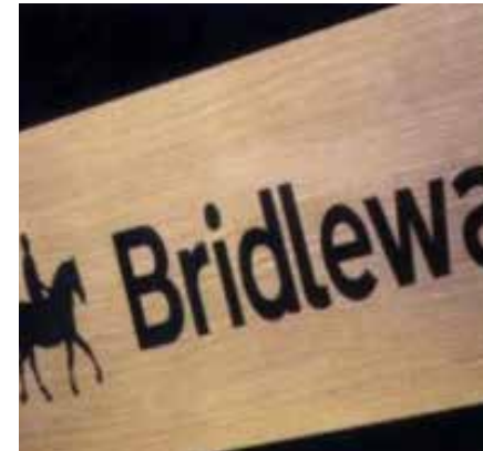
Above and below examples of laser cut text and icons in oak, back filled with resin paint.
