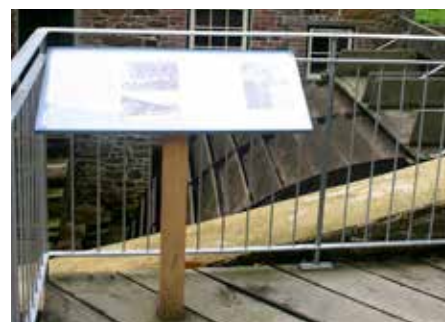
Above, PET grp panel with reverse print mounted to 18mm PVC back panel encapsulated in clear resin to protect against the 'salty' atmospheric conditions. Mounted on a seasoned oak post with galvanised steel brackets.
