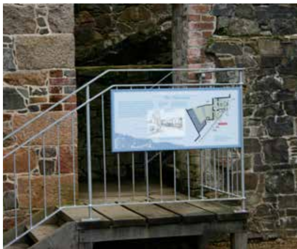
Above, PET grp panel with reverse print mounted to 18mm PVC back panel encapsulated in clear resin to protect against the 'salty' atmospheric conditions. Fitted to galvanised steel railings.
