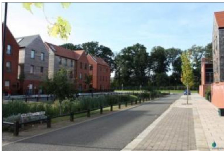
Figure 37 – Example of swale in residential street (SUSdrain, 2013)
