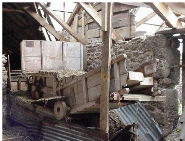
A now rare fixed thresher powered from the adjacent round house (horse engine house). © Philip White
