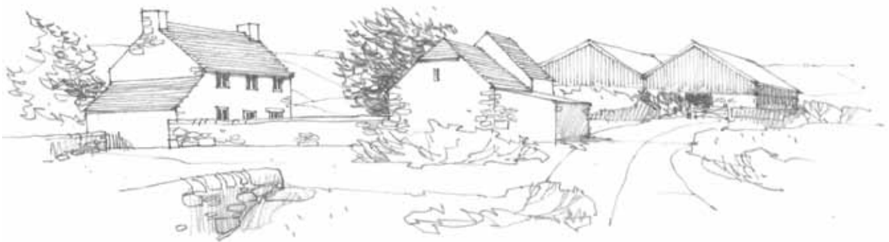
Breaking the roof and minor repositioning behind existing buildings or trees can help to reduce the visual impact even in prominent views
