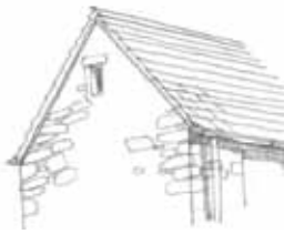
Verge and eaves should be plain and simple, tight to face of the walls
