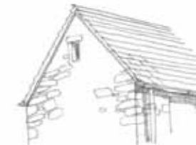
Verge and eaves should be plain and simple, tight to face of the walls
