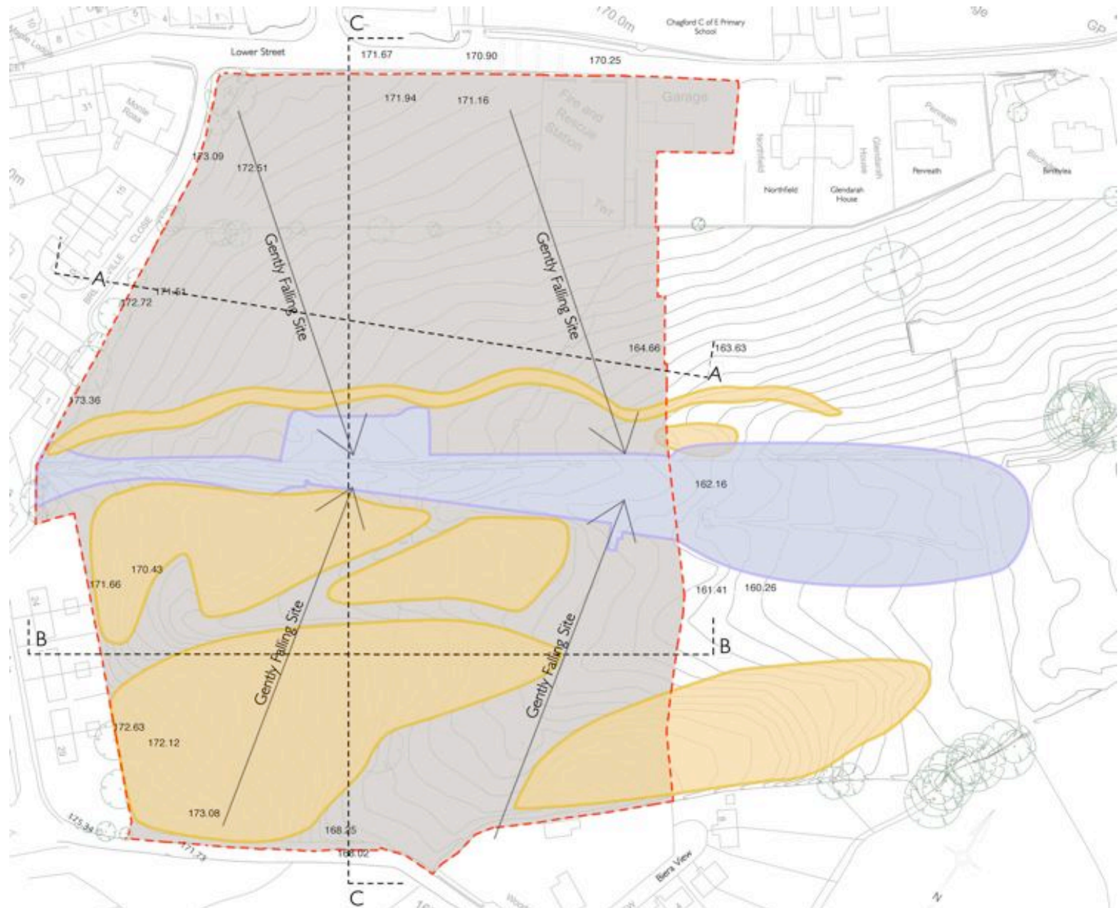
Fig.31 Existing Site Levels Plan Extract from 912/SK410 Proposed General Site levels NOT TO SCALE
